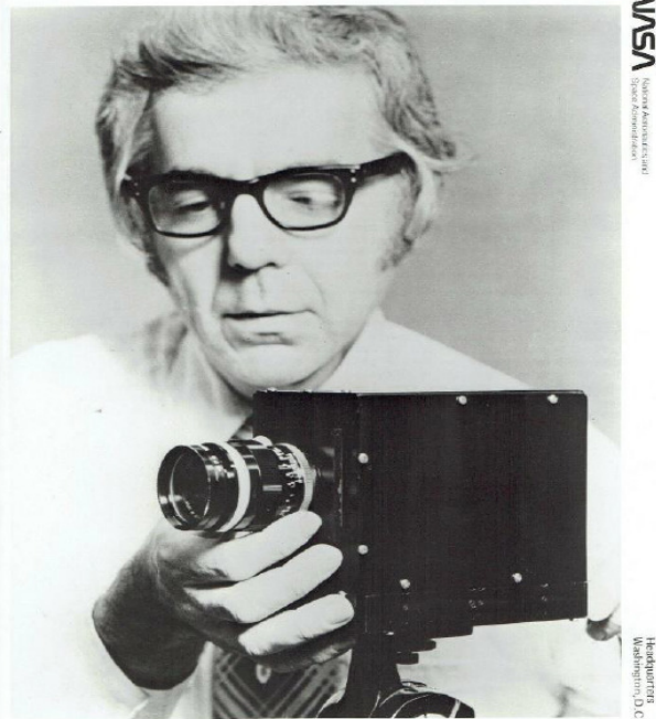
1976 Original Photo by NASA RCA Program Manager adjusts tubeless Space TV camera
